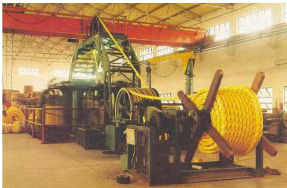
Production of 8-strand Mooring Rope
